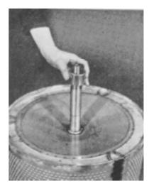
13. Fit two sealing rings from the inside of the wall and a seal from the outside of the wall. First lubricate the seals with a little grease.
