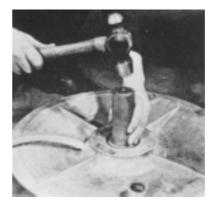
14. Fit the entry sleeve to protect the sealing rings when the rear wall is fitted.
