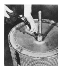
12. Heat the new bushing to approximately 150°C with the aid of a hotplate, an oven or similar device. Fit the bushing to the shaft.
