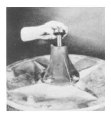
21. Fit the sealing ring and the flat key.
