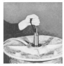
19 Pack grease around the shaft and then fit the bearing housing. Tighten the bearing housing bolts. N.B. Washers.
