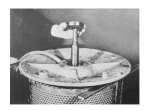
17. Fill the front bearing with grease and grease the bearing surfaces a little. Put the front bearing on the shaft and knock it into position in the rear wall. Remove the bars and knock the bearing into position on the shaft.
