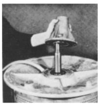
20. Grease the rear bearing and fit it on the shaft.
